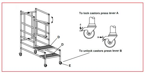
Fit small platforms (D) to form steps up to the top platform. Ensure the locking mechanisms of the hooks have engaged.
