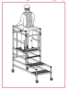
When on the platform ensure swinging braces are fitted correctly as shown, and gate is also closed.
