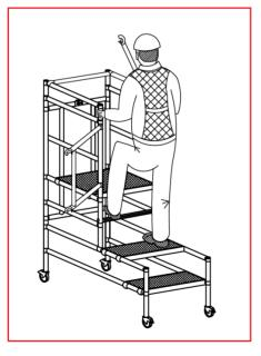
Climb up on to the platform using steps and climbing rung. To descend climb down as shown in diagram to the left.
