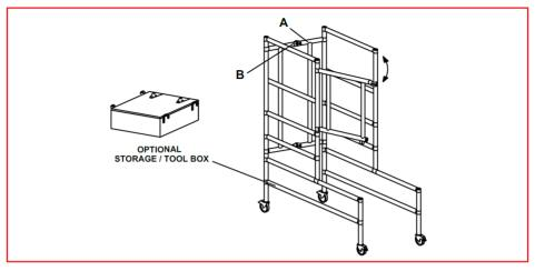
Open steps until folding frame (A) mechanisms lock automatically at (B)
