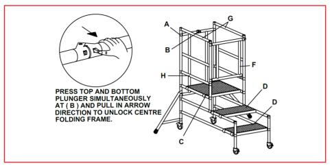
Fit work platform (C) at required rung height.
