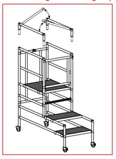
Fit adaption Kit to top of frame ensuring that the clip pins engage in the holes of the spigots. Also fit climbing rung.
