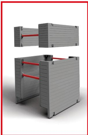
The Backhoe Manhole Box is a four-sided excavation box which provides a safe working area below ground. The Backhoe Manhole Box can sustain earth pressures of 20kN/m<sup>2</sup>. Users should check that the excavation will impose no greater pressures than this.
