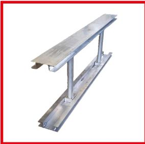
The Gen Shore Vertical Frame (GSVF) is a manually installed, hydraulically operated trench support system. The system is used for the short-term support of narrow and shallow trenches up to 2.0m wide x 2.0m deep in good ground that is stable, non-water bearing and capable of compression. The frames are used in sets of 3 and installed intermittently at 1.2m centres along the trench.
