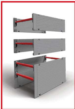
The Mini Trench Box can be used in trenches up to 4000mm deep with widths from 610mm to 3200mm, which can be altered using telescopic struts. Up to two extension boxes can be added on top of the mini Trench Box to achieve additional depth.
