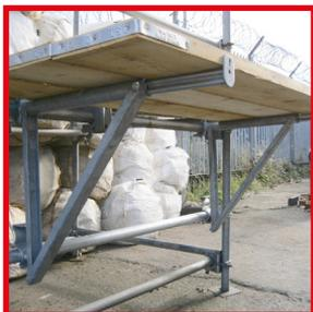
Altrad Generation Extendable Hop Bracket complements tube and fittings and Readylok Transoms. The bracket allows a two or three inside intermediate board platform to be constructed, also allowing the benefits of the speed of adaptation of the intermediate inside platform thus saving labour.
