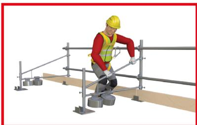
Altrad Generation's Safeguard System is approved to the Class A requirements for sloping roofs less than 10 degrees and additionally, as an added safety measure, we have tested and fulfilled the Dynamic Load Test to Class B of BS EN 13374:2004 to give further confidence for example, in the event of a person stumbling into the barrier.
