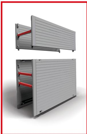
The Backhoe Trench Box is a robust piece of equipment, which acts as a safety shield to provide a safe working area below ground level. For use when working on excavations and pipe laying operations. The Backhoe Trench Box can sustain working earth pressures of up to 20kN/m<sup>2</sup>, users should check that the excavation will not impose greater pressures than this.
