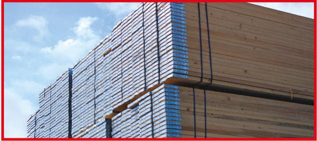
All our boards are made to the exacting standards of BS 2482:2009 using visually or machine graded timber with support spans of up to 1.2m or machine stress graded with support spans of up to 1.5m.
