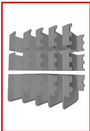
The Manhole Box is a four-sided excavation protection system, which is used whilst installing pre-cast manholes, chambers or tanks. The Manhole Box can be used in conjunction with trench boxes.
