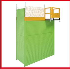
End panels are used in conjunction with Altrad Generation Trench, Manhole and Drag Boxes to safely seal off the open ends of an excavation and provide a completely enclosed working environment.
