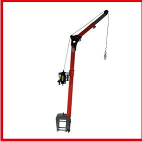
Altrad Generation Davit Arms' unique four piece construction allows single operative installation and ease of use on site. Allowing its manual rescue winch to easily lift upto 140kg from all types of box and sheeted excavations.
