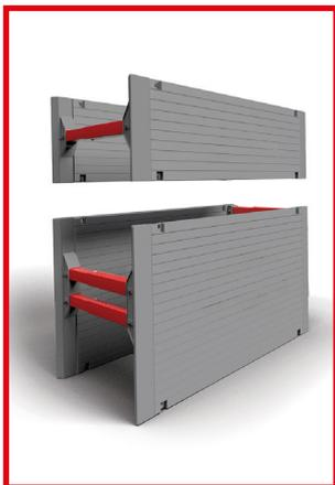
The Drag Box acts as a shield to protect users in self-supporting soil. It is designed to withstand up to 25kN/m<sup>2</sup>. Installation requires the 'Excavate and Drag' technique, the box is placed in a pre-dug trench and moved after each instalment of pipe.
