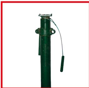
Available stock in four sizes, Altrad Generation's Trench Struts feature clawed base and head plates to enable a better grip to the trench lining and hold it tightly in place preventing collapse. All struts are manufactured to BS4074:2004 and are thread rolled to ensure there is no cutting away of material or loss of strength.
